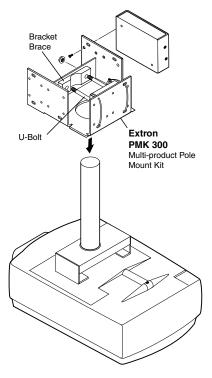
Figure 2-6 — Projector pole on the inside
